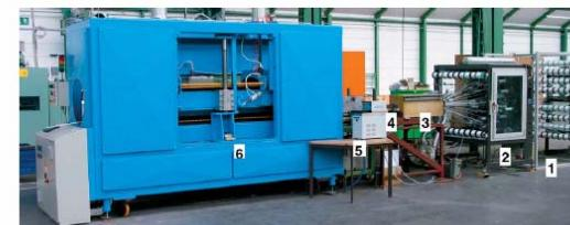
Fig. 13. ITV-braid pultrusion: reel for core- and axial-yams (1), brazier with heating yams (2), preheating device (3), heated die (4), water cooling
