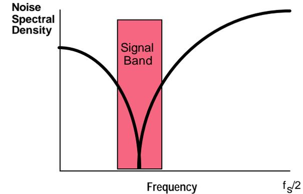
**The Noise Suppression Region Can Be “Tuned” Away From DC By Replacing The Lowpass Filter With A Bandpass Filter**
