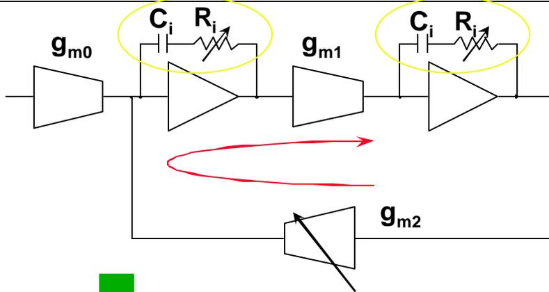
Frequency and Q can both be tuned by varying a gm
