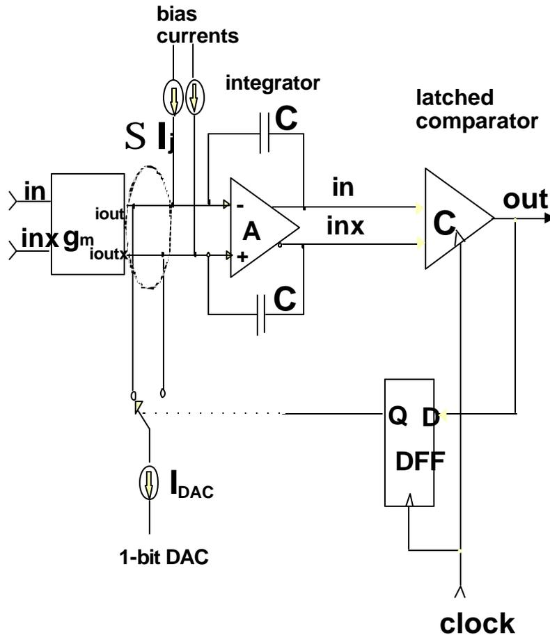
**Basic Approach: High impedance current drive in a feedback integrator**
