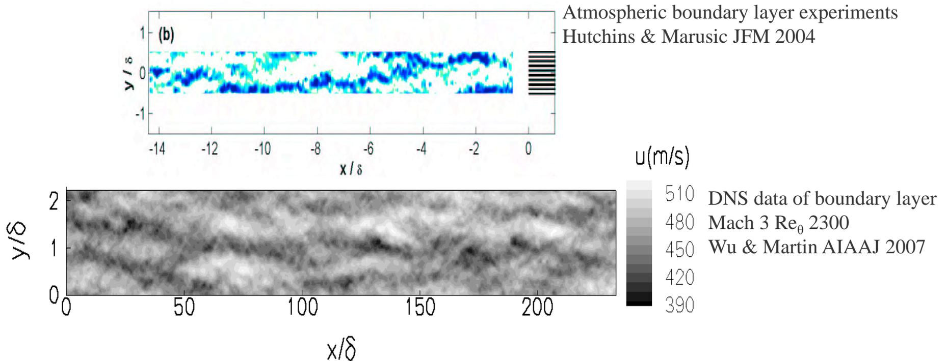
Rake signal from DNS data at  $z_n=0.2\delta$
