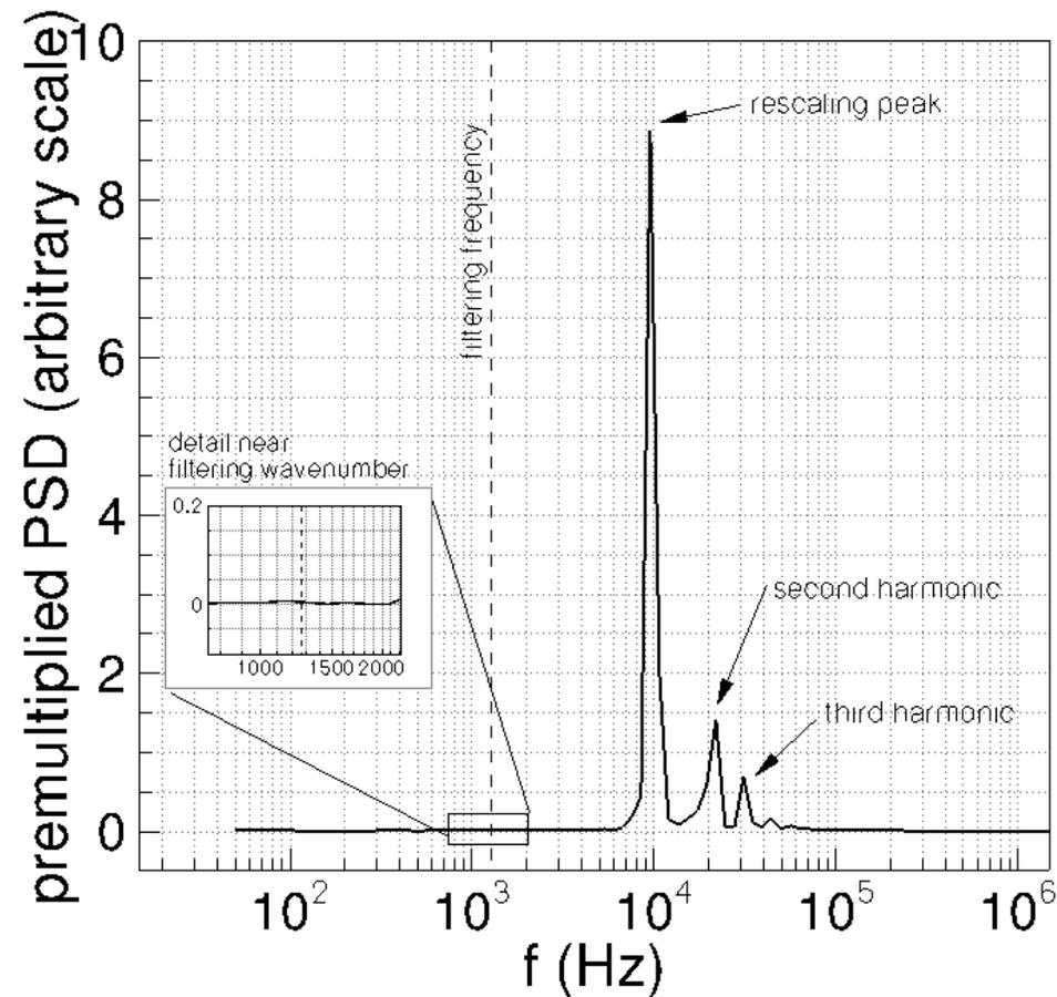
The filtering does not introduce any forcing in the flow.
