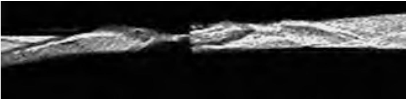
Flow inside a generic scramjet engine, no combustion
